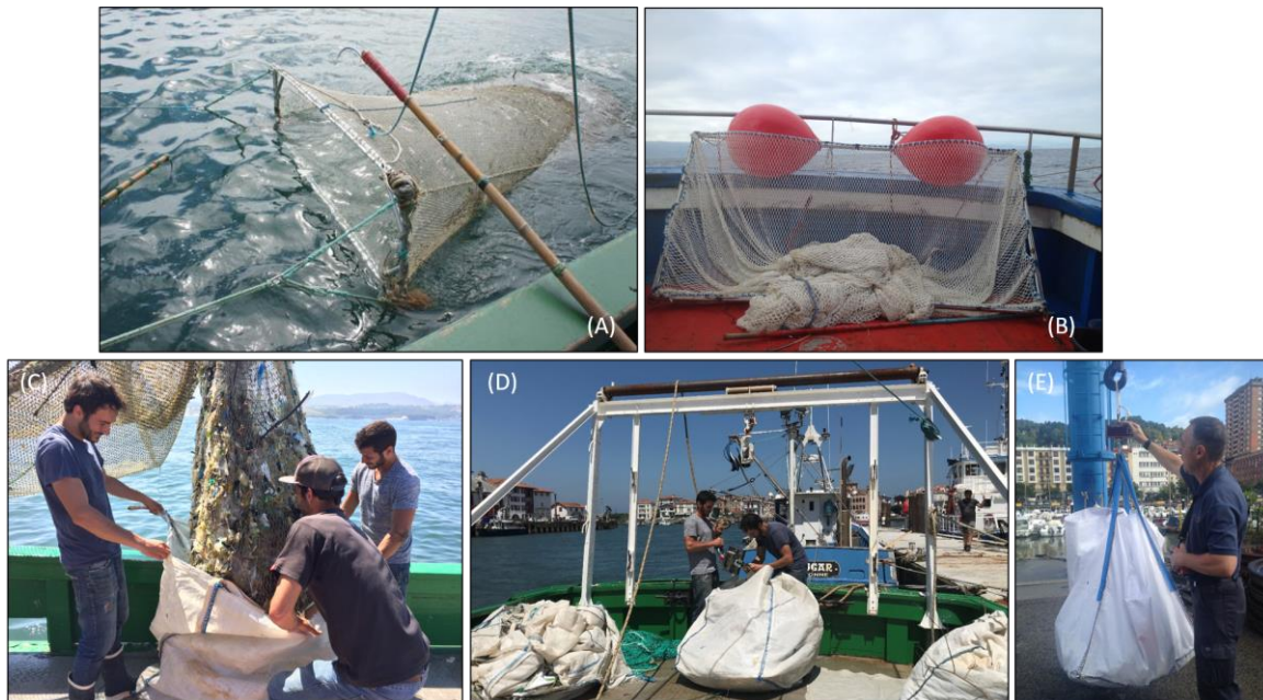
Figure 3 : FML collection gears used by the LEMA fishing vessels (A - Itsas Belhara, B - Miren Argia), storing FML in big bags onboard (C- example of the Itsas Belhara), and the weighting procedure onboard (D - Itsas Belhara), or in port (E - Miren Argia).
