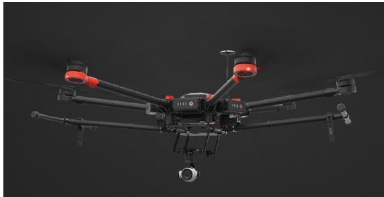
Figure 13: Zenmuse Z3- matrice 100 UAV system used for the experimentations
