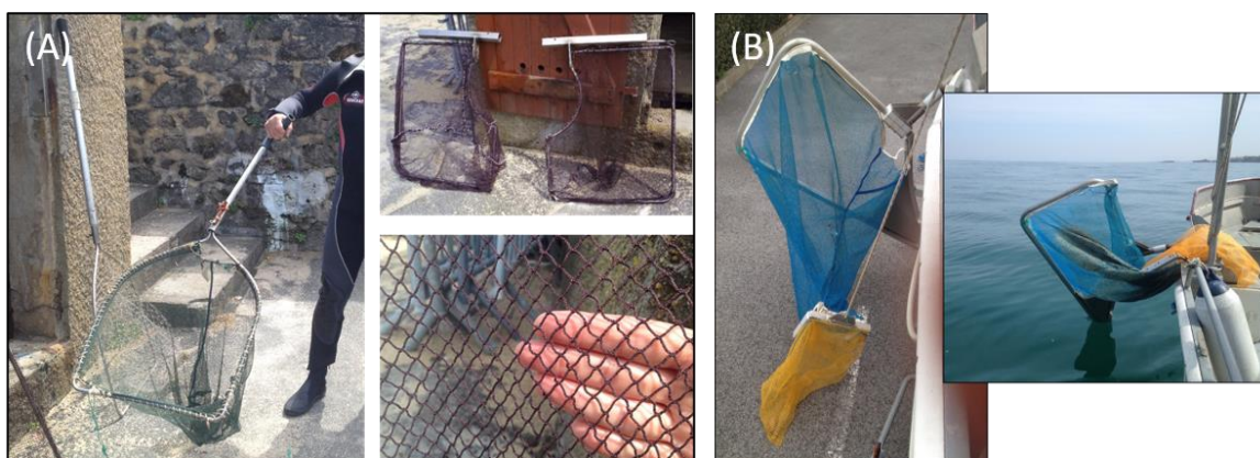
Figure 4 : Gears employed by the BAB Subaquatique (A) and the Uhaina (B) sea-cleaning vessels for collecting FML
