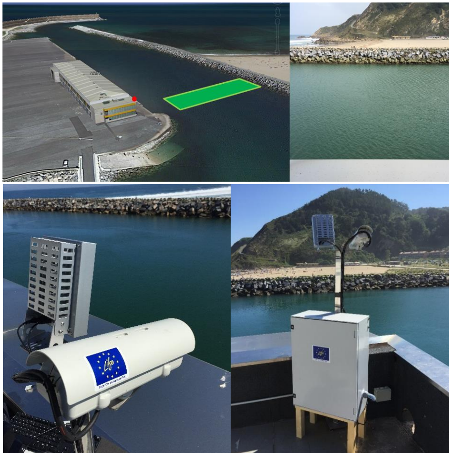
Figure 11: Illustrations of the Orio river video monitoring station
