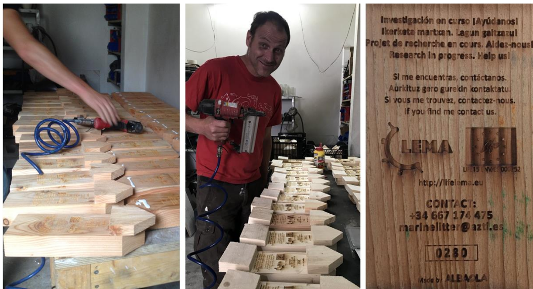
Figure 15 : Process of assembling pieces performed by Jenő Kocsis (local craft man) and example of laser printing
